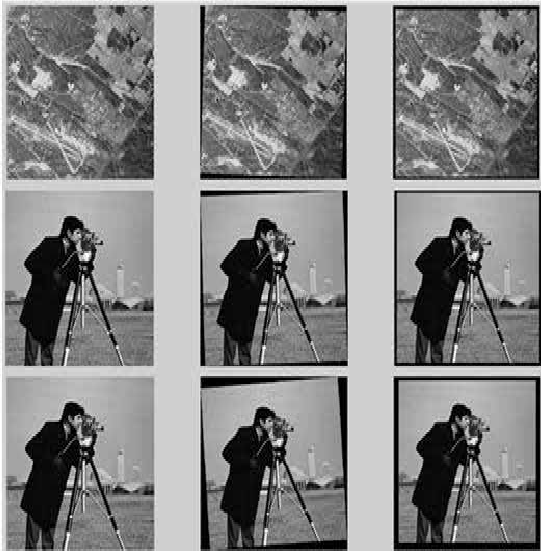
Figure 3.2 in each image dataset, first image is original, second image is generated by applying known rotation and third image is de-rotated by histogram based MI method after finding the rotation
